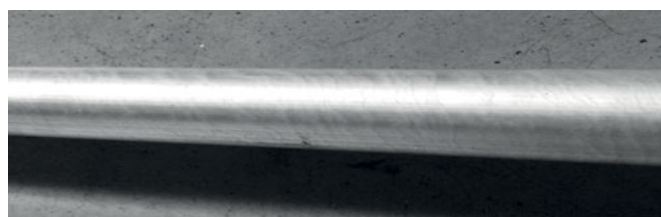
Fig.2. Surface of Mg alloy rod after on-line cooling
