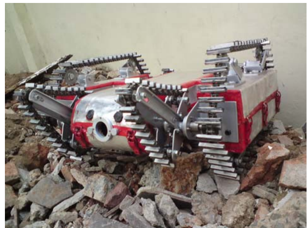
Fig. 1. CAESAR robot being tested on rubble
