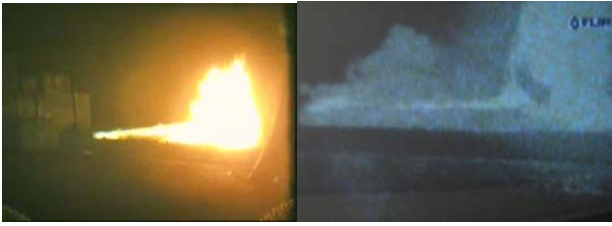
Fig. 14. The flame from a normal camera compared to a thermal camera
