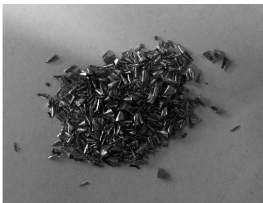
Fig. 6. Form of Cu-Zn44 alloy chips
