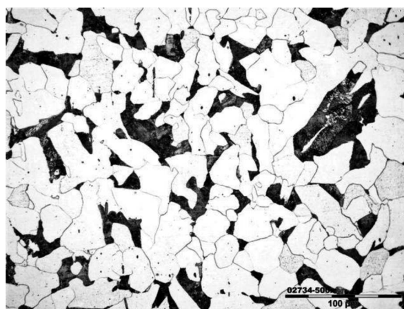
Fig. 6. ST3S steel - fine-grained ferritic-pearlitic structure (magnification of 500x)
