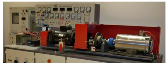
Figure 8. Machine test bench together with the proposed motor
