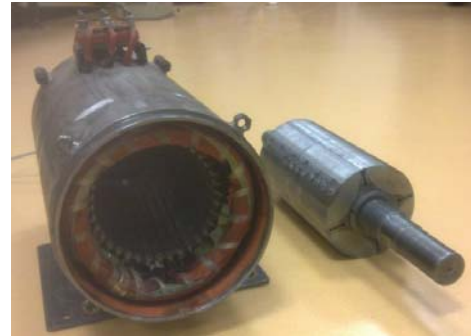
Figure 7. The prototype of the motor body and axially laminated rotor structure
