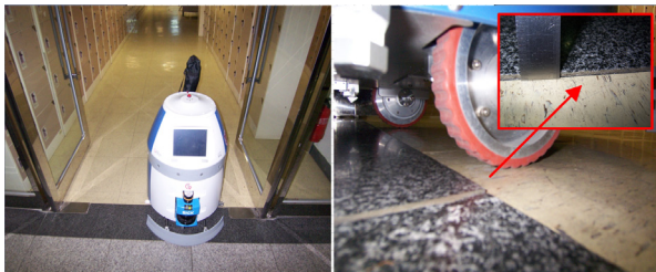
Fig. 12. Wheel slippage situation due to uneven floor condition.
