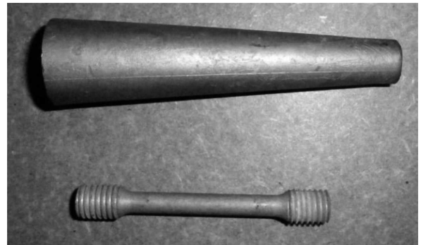
Fig. 3. Cast and sample for creep test
