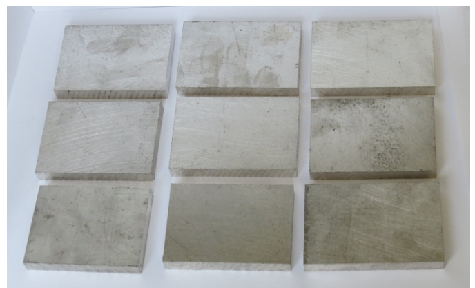
Fig. 6. Photograph of a selection of AZ31 alloy specimens used in the experiment
