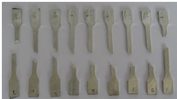
Fig. 14. Test specimens after fracture
