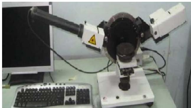
**Figure 2.** Ellipsometry with computer.
