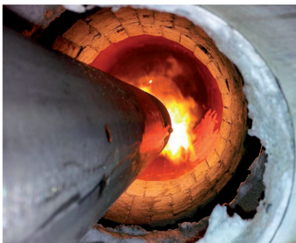
Fig. 2. Rotary kiln equipped with oxygen burner
