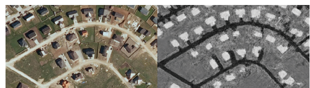
Figure 5. A sample image of suburban terrain (left) and its cost map (right). Dark colours on the cost map correspond to easily traversable areas (roads) and light colours are obstacles (buildings)
