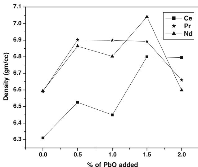
**Figure 3.** Variation of sintered density with respect to % of PbO addition.
