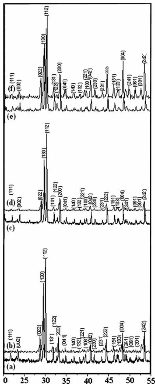
**Figure 1.** XRD patterns of (a) pure  $\text{CeTiTaO}_6$ , (b) 2%  $\text{PbO}$  added  $\text{CeTiTaO}_6$ , (c) pure  $\text{PrTiTaO}_6$ , (d) 2%  $\text{PbO}$  added  $\text{PrTiTaO}_6$ , (e) pure  $\text{NdTiTaO}_6$  and (f) 2%  $\text{PbO}$  added  $\text{NdTiTaO}_6$ .
