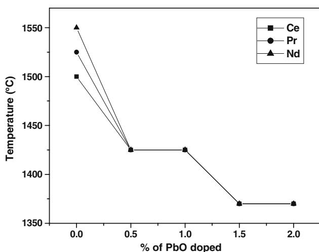
**Figure 2.** Variation of sintering temperature of  $\text{LnTiTaO}_6$  ceramics with % of PbO addition.
