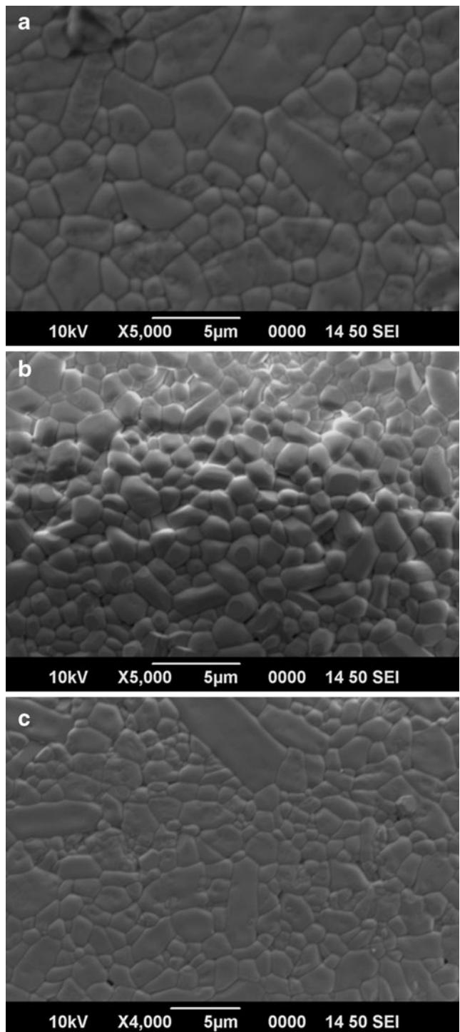
**Figure 4.** SEM images of 1 wt% PbO added **a.**  $\text{CeTiTaO}_6$  ceramic, **b.**  $\text{PrTiTaO}_6$  ceramic and **c.**  $\text{NdTiTaO}_6$  ceramic.
