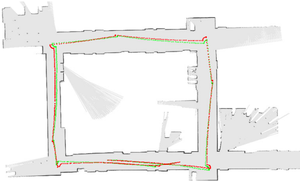
Figure 8. The robot trajectory estimated by PFOI with only 5 particles. The red one is the ground truth (approximate) and the green one is estimated by PFOI.
