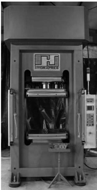
Fig. 5. Hydraulic press, max force 250T
