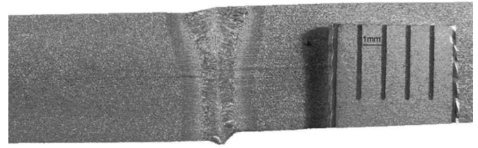
Fig. 5. The cross section of Yb:YAG laser butt-welded joint
