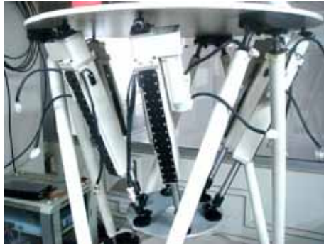
Figure 5. The telescopic drive PKM
