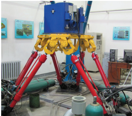
Figure 3. Experimental electro-hydraulic parallel manipulator
