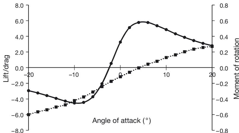
Fig. 3. Lift/drag ratio (solid line) and pitching moment of rotation about the centre of gravity (dashed line) of the models versus the angle of attack during steady gliding calculated in the computational fluid dynamics analysis. The moment of rotation was divided by the mass of the body times the flow velocity squared and is dimensionless
