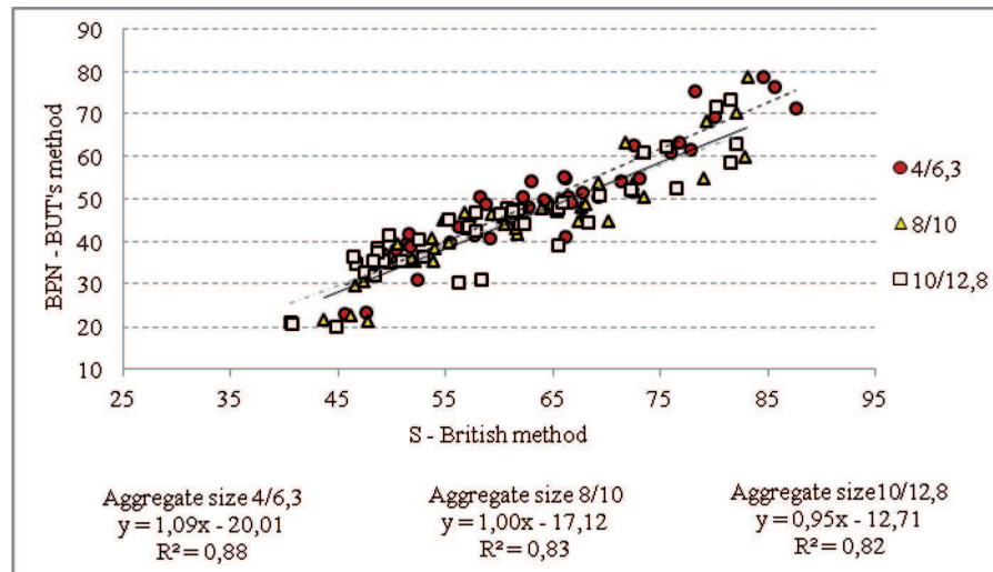
Fig. 5. Relation between the BPN and S values depending on the grain size of aggregates.
