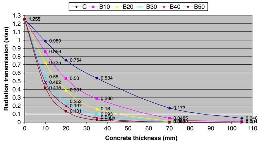
Figure 7. X-ray 150 kV (118 keV) measurement results of the concretes.
