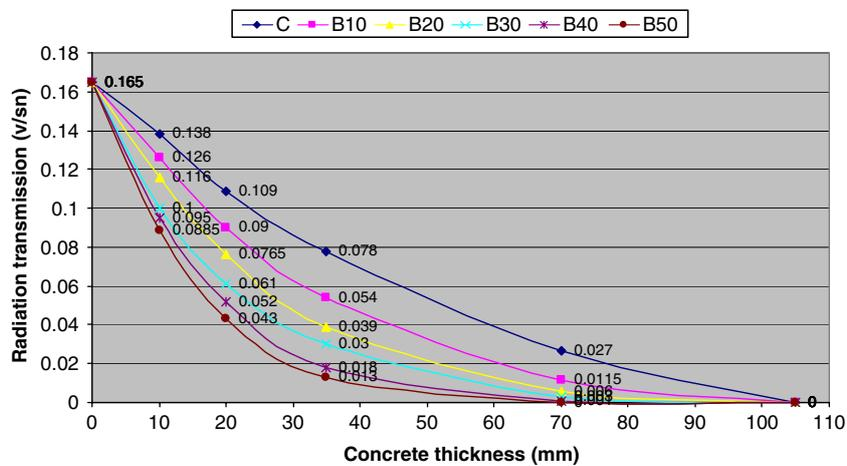
Figure 8. X-ray 200 kV (164 keV) measurement results of the concretes.
