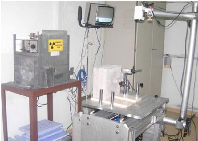
Figure 4. Cesium measurement device.
