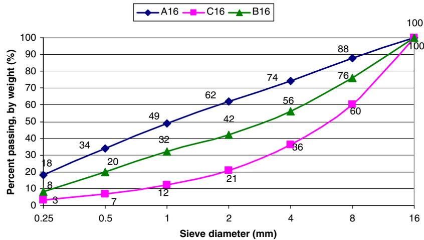
Figure 1. Granulometry curve of the aggregates used in the experiments.
