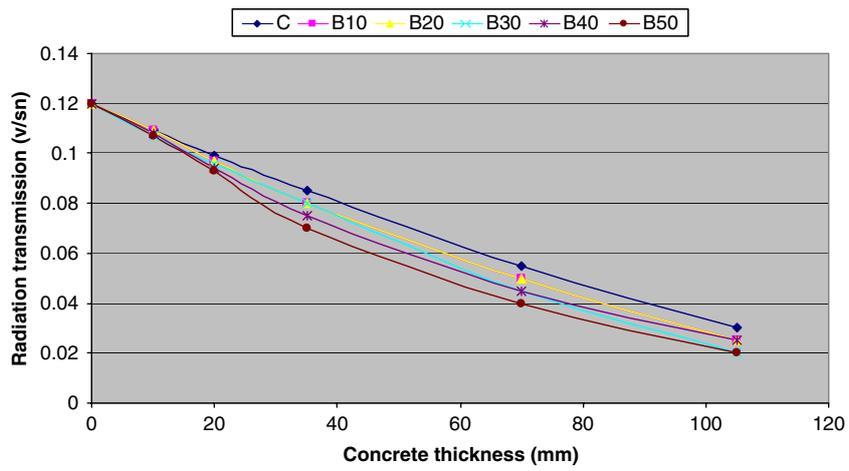
Figure 9. Cs-137 ray (662 keV) measurement results of the concretes.
