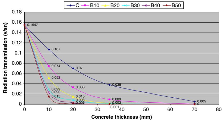
Figure 6. X-ray 100 kV (85 keV) measurement results of the concretes.
