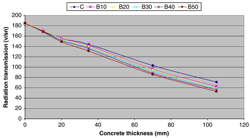
Figure 10. Co-60 ray (1250 keV) measurement results of the concretes.
