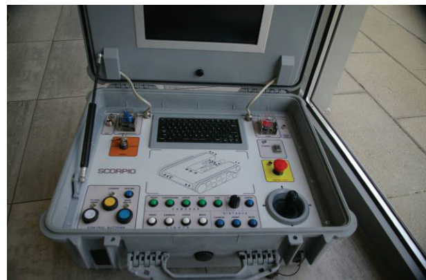
Figure 2. The wirelessly connected portable briefcase remote control device with control panel of the service robot SCORPIO
