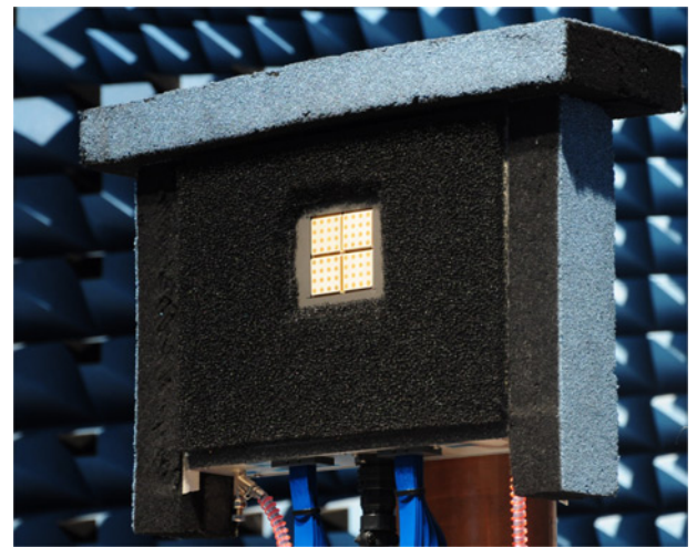
Fig. 6 8 \times 8 Rx array mounted on the manifold in an anechoic chamber
