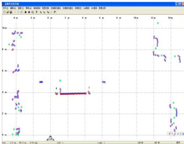
Fig. 5 Data clustering and feature extraction of one laser sensory frame
