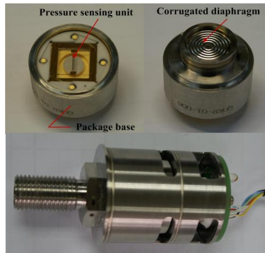
Figure 5. The packaged pressure sensor.
