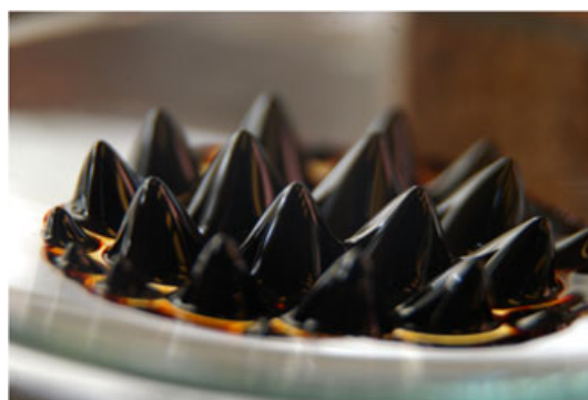
Figure 6. A 50 wt% aqueous ferrofluid solution of carboxysilane-coated NPs stabilized by electrostatic repulsion with a magnet underneath.
