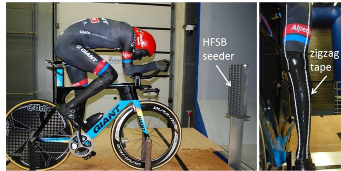
Figure 1. Cyclist and HFSB seeding system (left) and the application of zigzag tape on the stretched leg (right).
