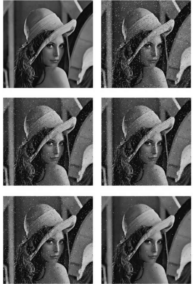
Fig. 3 Results of denoising obtained with Lena image (variance of salt and pepper = 0.04). From left- to right-hand side and from top to bottom: result of [21] algorithm, result of [22] algorithm, result of [17] algorithm, and result of the new algorithm
