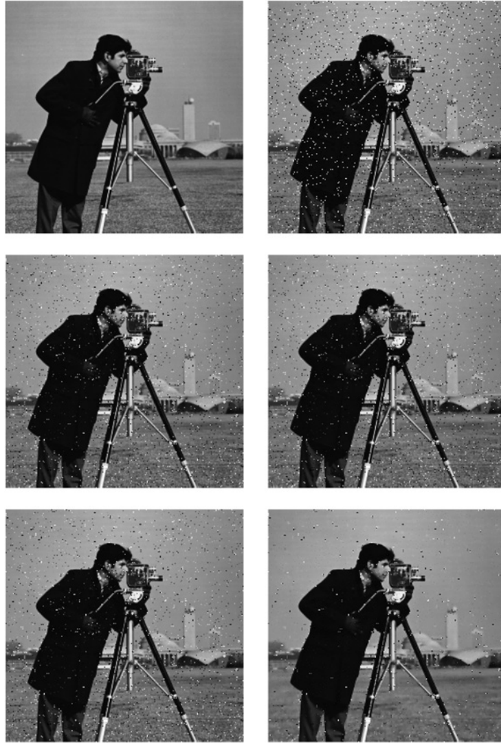
Fig. 4 Results of denoising obtained with Cameraman image (variance of salt and pepper noise = 0.04). From left- to right-hand side and from top to bottom: result of [21] algorithm, result of [22] algorithm, result of [17] algorithm, and result of the new algorithm
