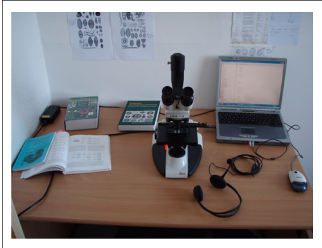
Figure 1. Equipment configuration, illustrating headset with microphone linked to a laptop computer running EcoCount.
