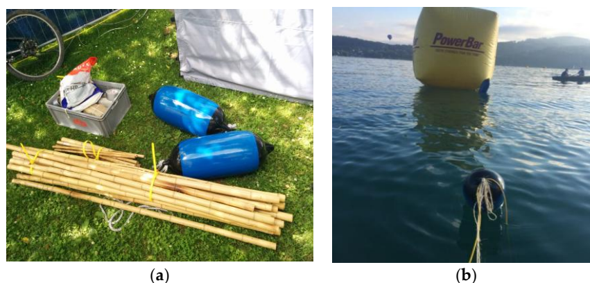
Figure 5. (a) Components of the underwater timing antenna; (b) Operation in the lake, view from the timing boat, in the background the yellow turning buoy, in the foreground the fender buoy.
