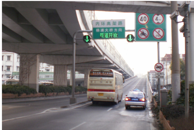
Figure 1. Arterial road variable message signs in Shanghai.
