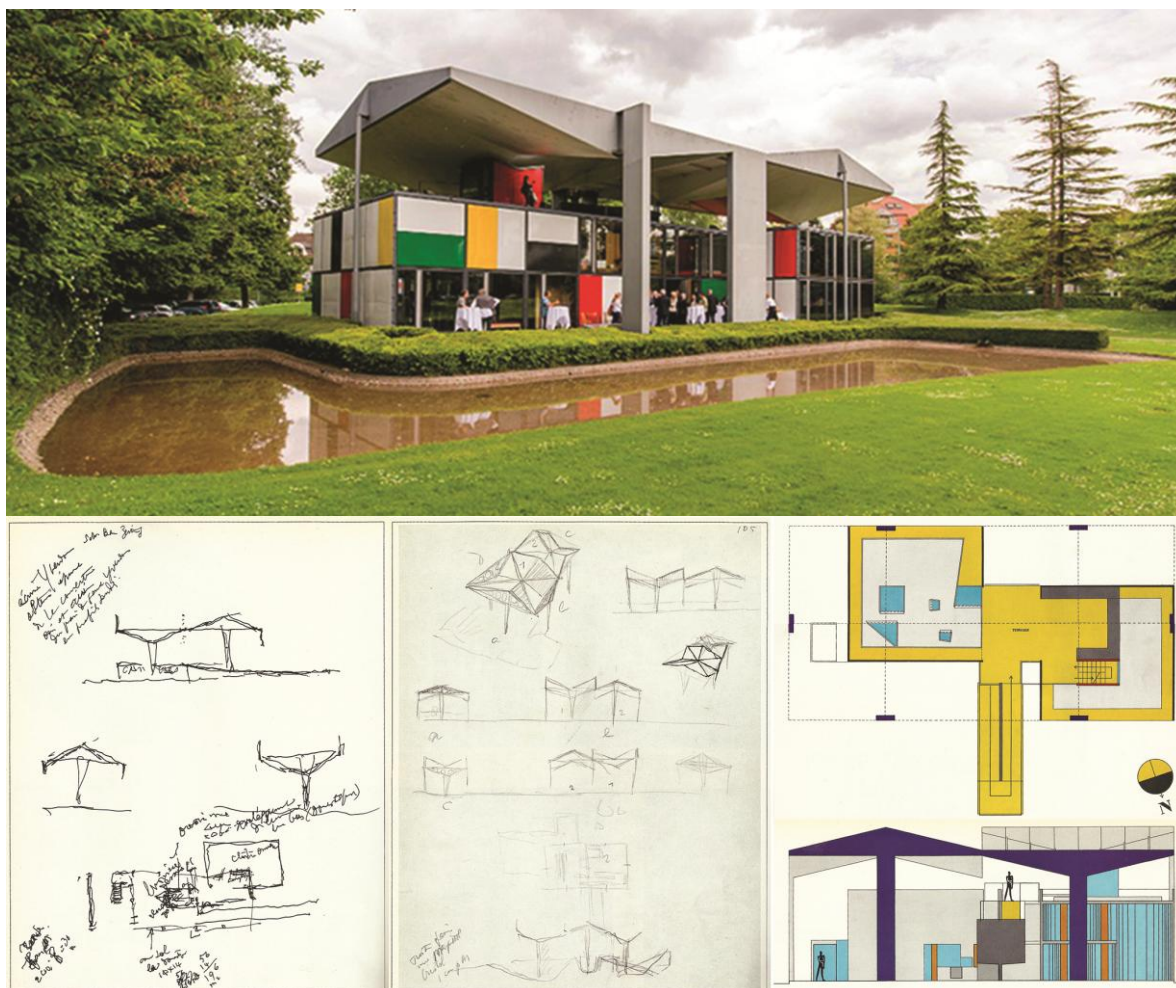
Figure 4. Pavillon Heidi Weber, Center Le Corbusier, Zurich. First sketches, studies on the geometries of the two covers and supporting pillars. The relationship between the roof structure and the architectural spaces - plant and section.
