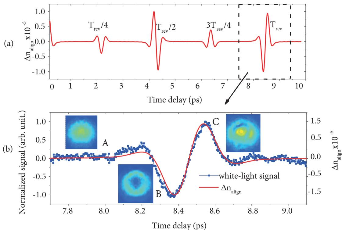
**Figure 2.** (a) The calculated periodic modulation of the refractive index induced by nonadiabatic molecular alignment, (b) the measured white-light signal around the full revival time of molecular nitrogen. The insets show the probe beam patterns (beam cross section) recorded by using the CCD camera at delay-A (randomly oriented molecules), delay-B (molecular antialignment), and delay-C (molecular alignment).
