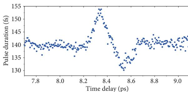
**Figure 4.** The measured pulse duration induced by the full revival of molecular alignment for nitrogen.
