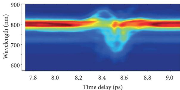
**Figure 3.** The measured spectral modulation around the full revival time of molecular nitrogen.
