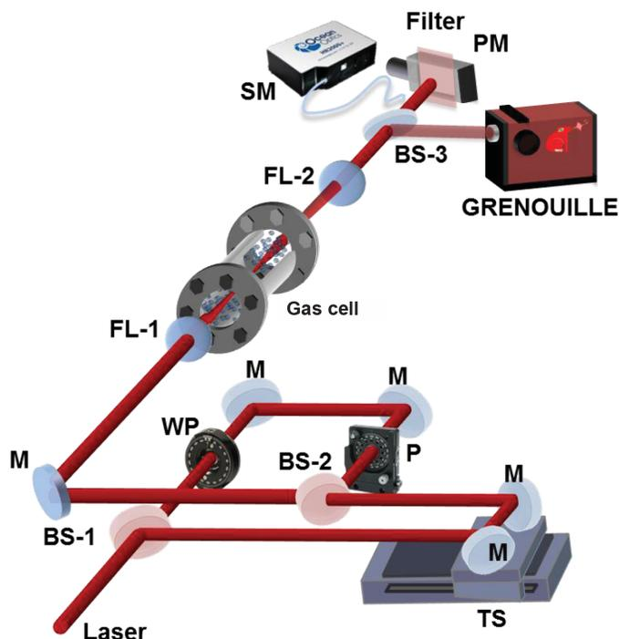
**Figure 1.** The schematic of the experimental setup. BS: beam-splitters, TS: translational stage, WP: wave plate, P: polarizer, M: flat mirrors, FL: focusing lens, SM: spectrometer, and PM: power meter.
