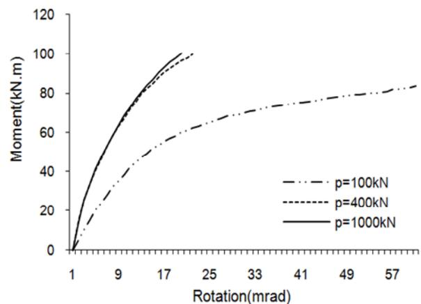
**Figure 5.** Moment-rotation curves resulted from the laboratory tests (Jaspart and Vandegans, 1998).
