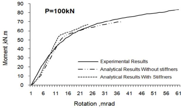
Figure 6. Comparison of the test results and numerical (Analysis for P=100 kN axial force).
