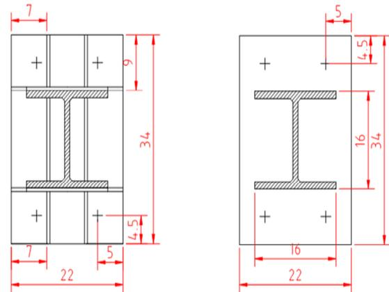
**Figure 4.** Column base plates used in the test and analysis.
