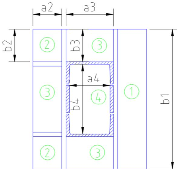
**Figure 1.** Different regions of a stiffened column base plate (Irani, 1996).
