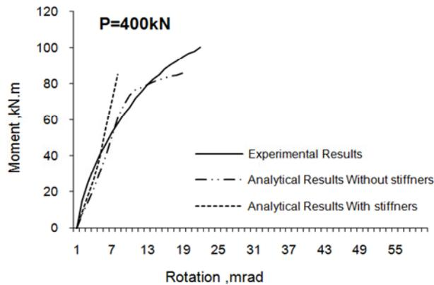
Figure 7. Comparison of the test results and numerical (Analysis for P=400 kN axial force).
