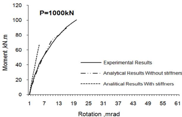
Figure 8. Comparison of the test results and numerical (Analysis for P=1000 kN axial force).
