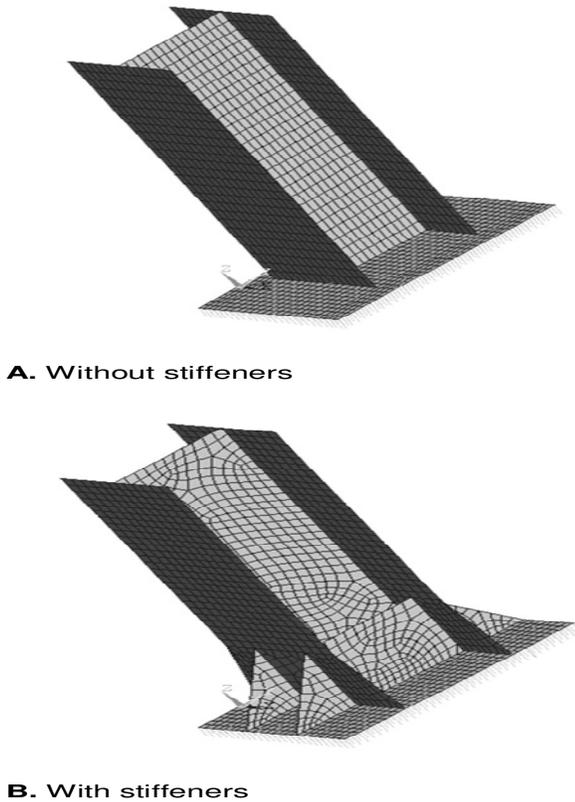
**Figure 3.** Analytical models of column base plate without and with stiffeners (axial force and moment).
