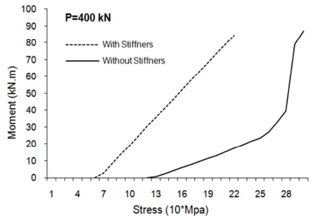
Figure 10. Noticeable effect of stiffeners on reducing flexural stresses.
