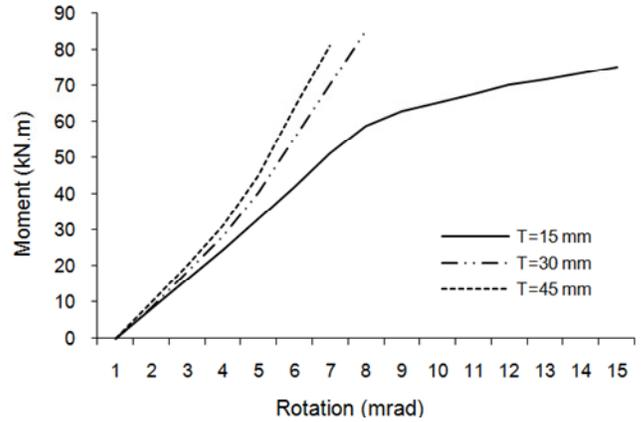
Figure 9. Effects of plate thickness on the connection rigidity.
