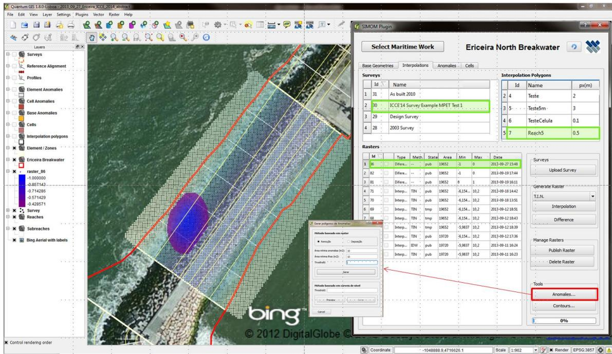
Figure 14. SIMOM – Ericeira North breakwater example of an anomaly identification using the QGIS plugin.
