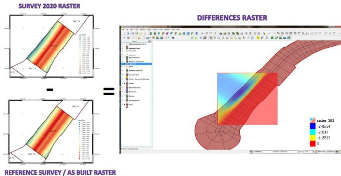
Figure 13. Comparison of two surveys rasters (left) to obtain a differences raster (right).
