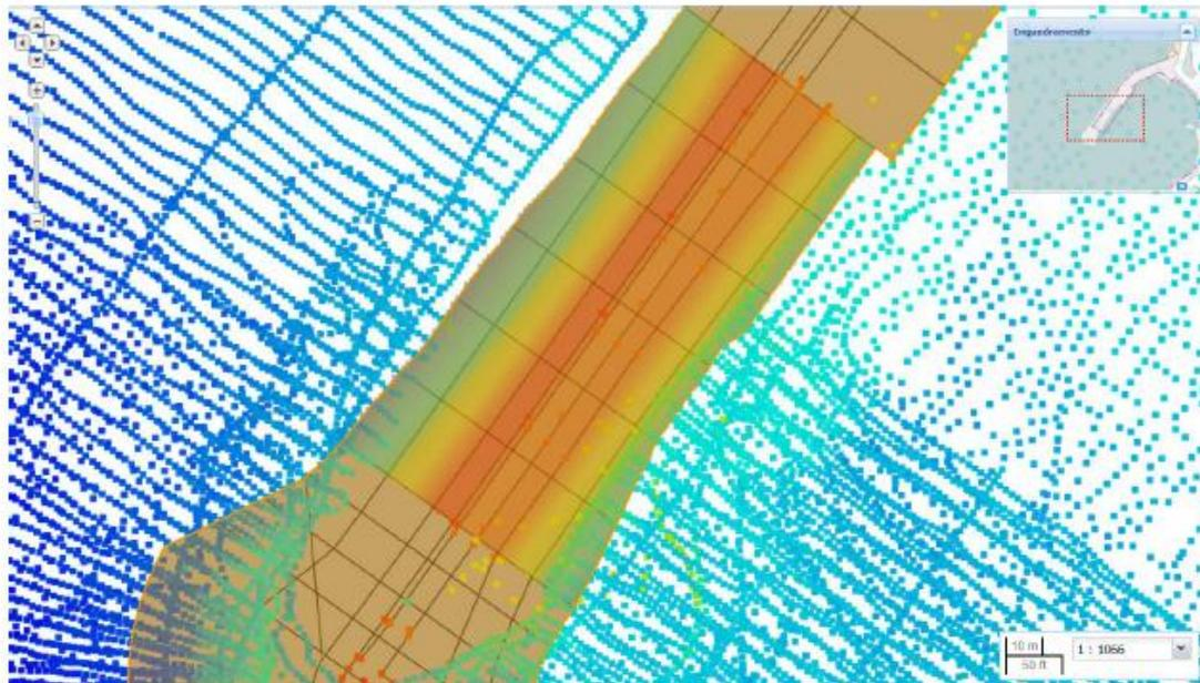
Figure 12. Survey example with variable resolution. This data will be used to interpolate to a raster file to allow condition performance.
