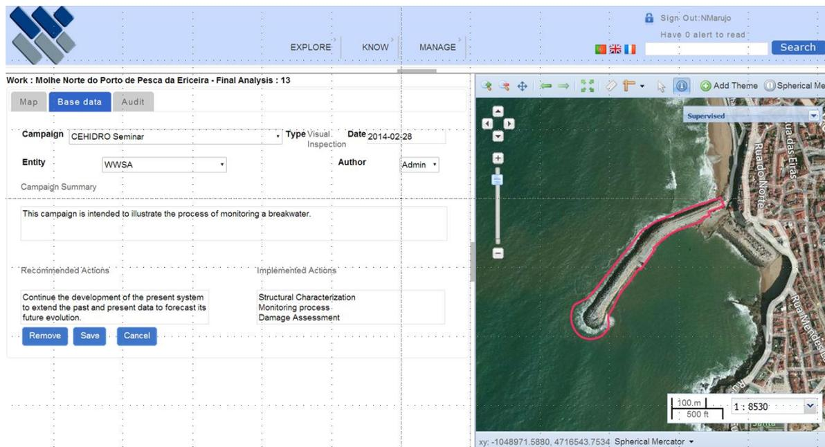
Figure 17. SIMOM – Ericeira North breakwater – example of the final analysis for a campaign including summary, recommended actions and implemented actions.
