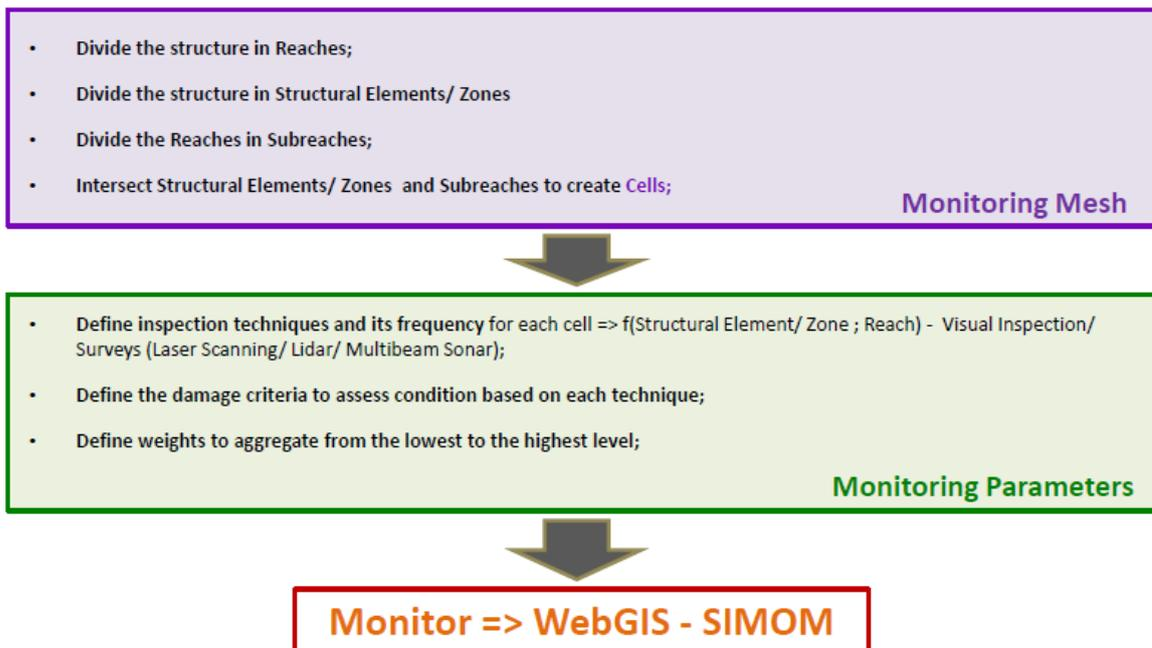
Figure 2. Monitoring methodology - Preparation phase.
