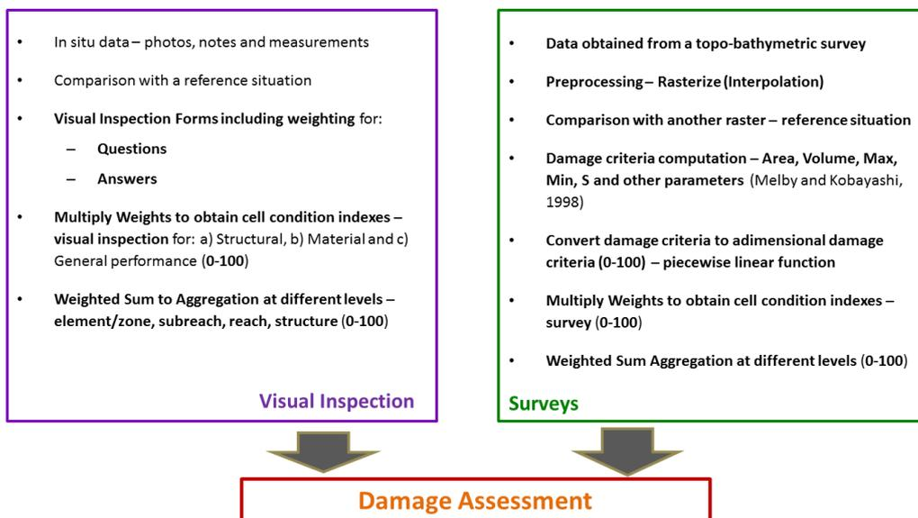
Figure 9. Comparison between visual inspection and survey based damage assessment
