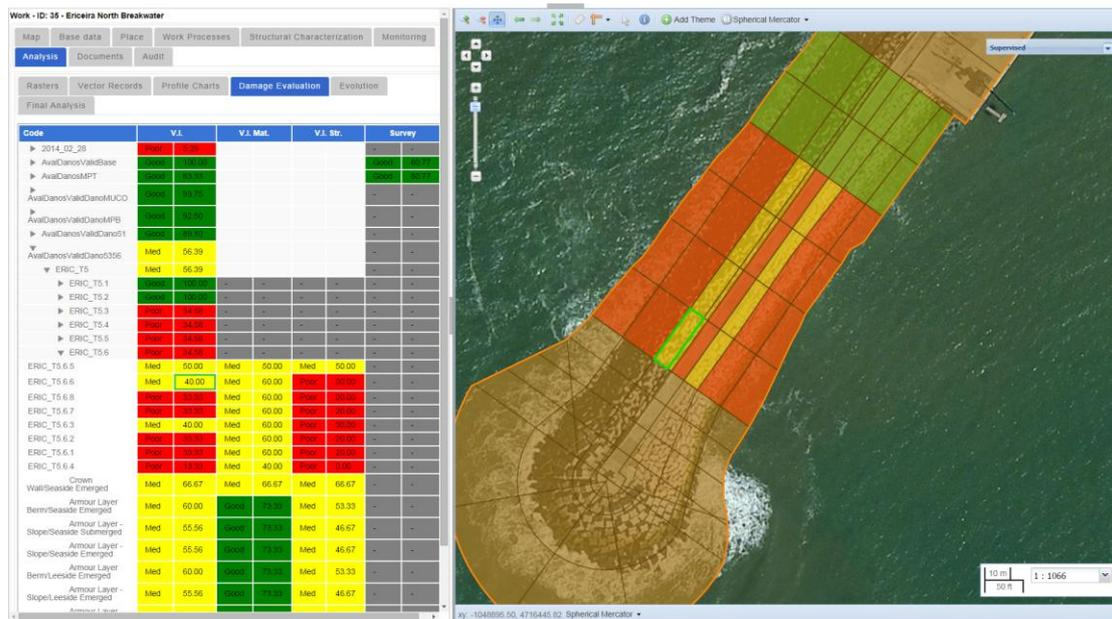
Figure 16. SIMOM – Ericeira North breakwater example of cell condition levels in the case subreaches 5.1 and 5.2 are not damaged and some severe damage may be found in subreaches 5.3-5.6 especially in the armor layer and pavement. Condition levels at the different assessment levels: campaign, reaches, subreaches, structural elements/ zone and cells (left) and map representation of these condition levels for cells in geometry (right).
