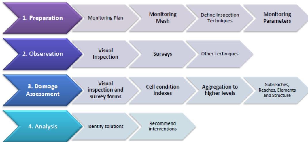
Figure 1. Monitoring methodology including 4 phases: preparation, observation, damage assessment and analysis.
