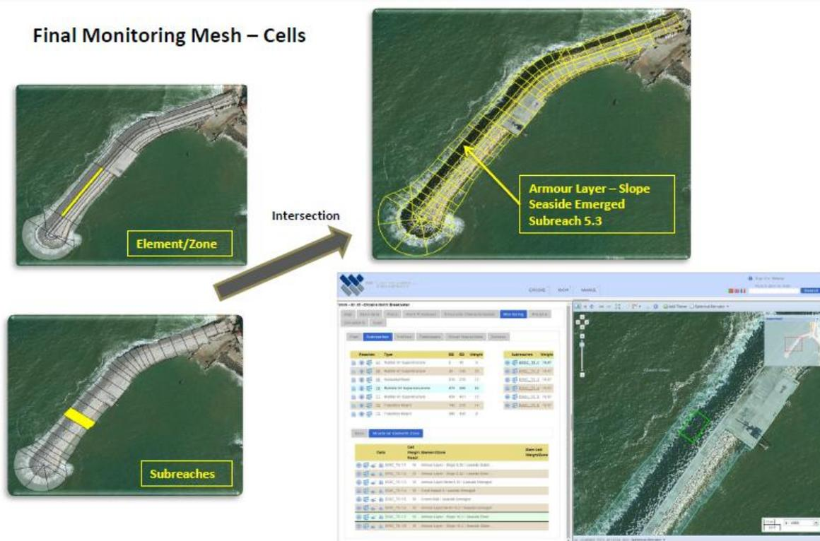
Figure 8. Ericeira North breakwater monitoring mesh and highlight of a cell in SIMOM.
