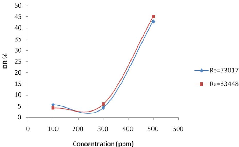
**Figure 5.** Relationship between iron particle concentration and percentage of DR for size particle 45 µm at Re = 73017 and Re = 83448.
