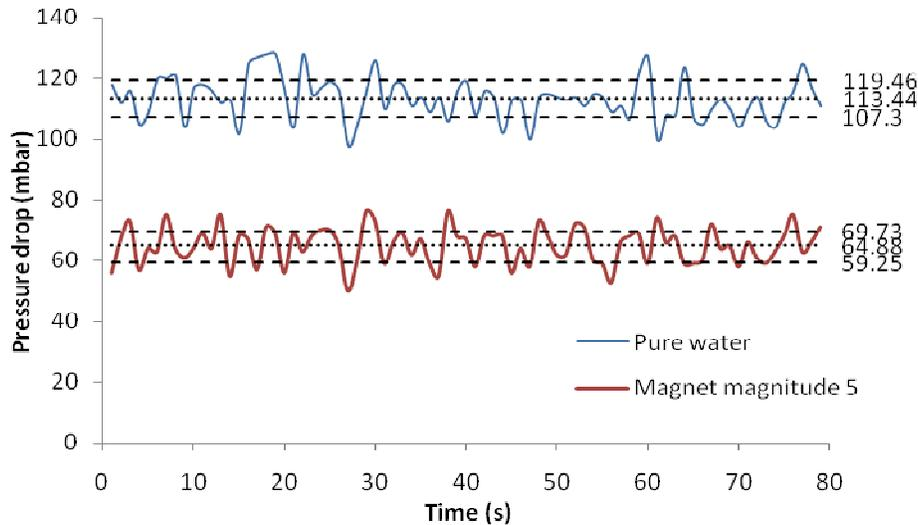
**Figure 9.** Behavior of the pressure drop influenced by the magnetic field applied for iron particle 45  $\mu\text{m}$  of concentration 500 ppm at  $\text{Re} = 93879$  (compared with pure water).
