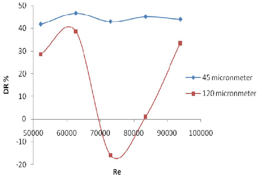
**Figure 7.** Relationship between iron particle size and percentage of DR for concentration of 500 ppm.
