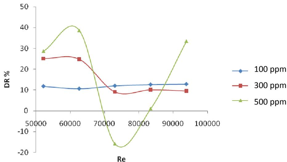
**Figure 4.** Relationship between iron particle concentration and percentage of DR for size particle 120  $\mu\text{m}$ .
