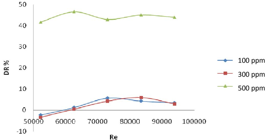
**Figure 3.** Relationship between iron particle concentration and percentage of DR for size particle 45  $\mu\text{m}$ .
