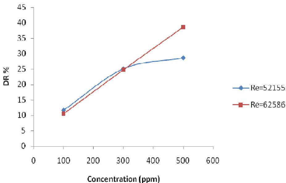
**Figure 6.** Relationship between iron particle concentration and percentage of DR for size particle 120 µm at Re = 52155 and Re = 62586
