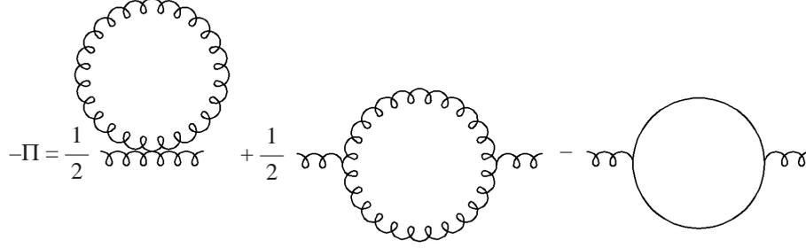
**Figure 1.** One-loop diagrams for gluon self-energy. Wavy and solid lines denote gluons and quarks, respectively.
