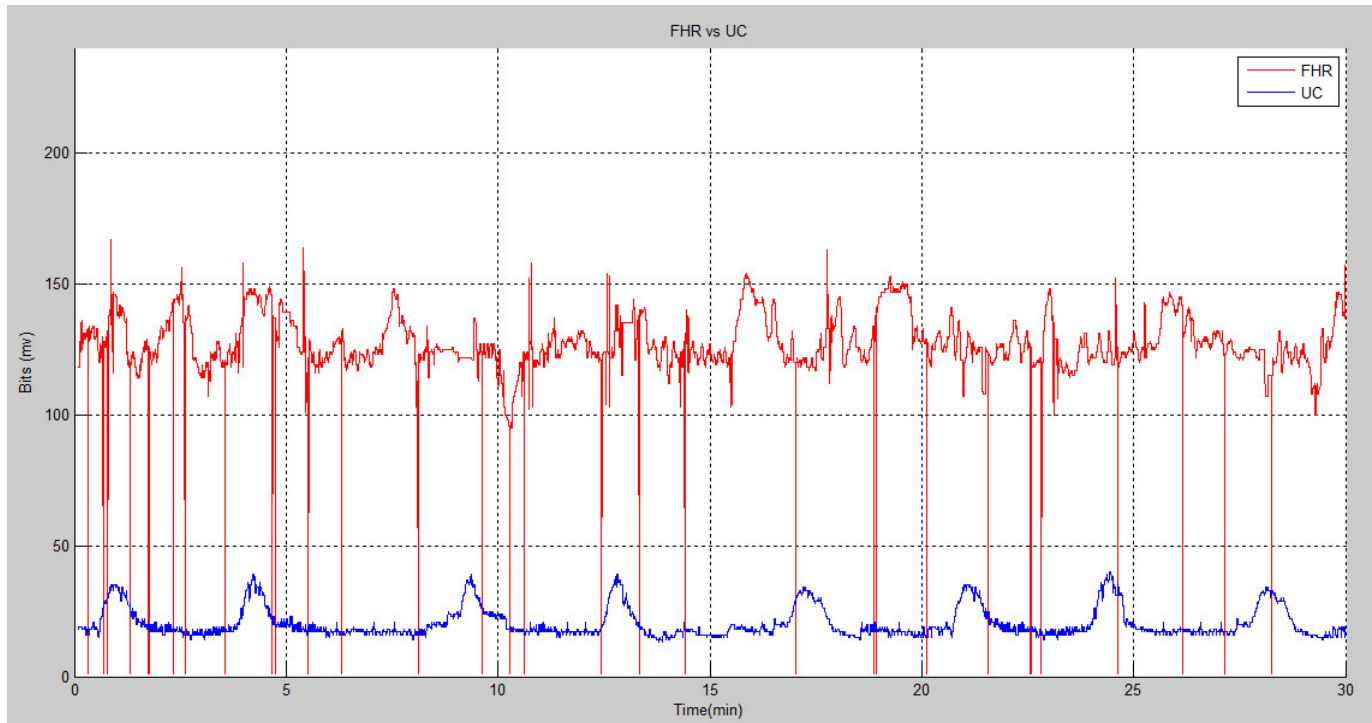
Figure 3a. CTG signal before pre-processing. The processing of CTG signals is to remove the spiky unwanted signal by using the low-pass filter and compensating the missing data during the process of measuring the data from the pregnant mother using the linear interpolation method for missing data compensation. Figure 3b shows the FHR signal after the pre-processing.
