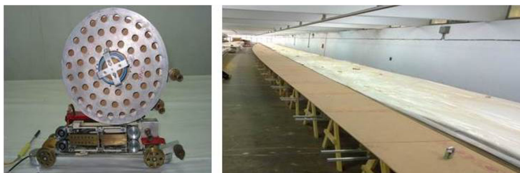
Fig. 5. The sealing machine (left) and curved table (right) used in balloon fabrication.
