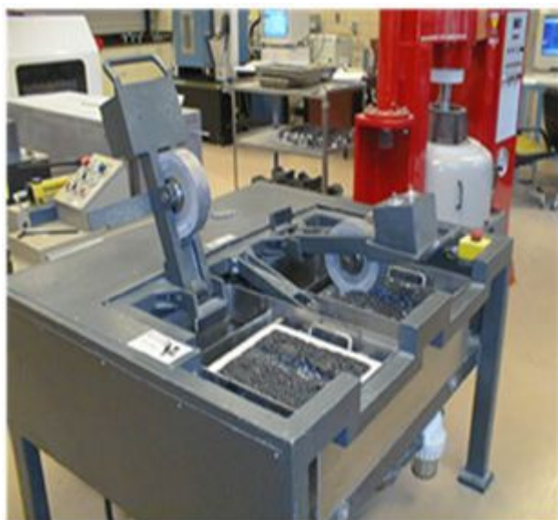
Figure 6. Wheel tracking test machine.
