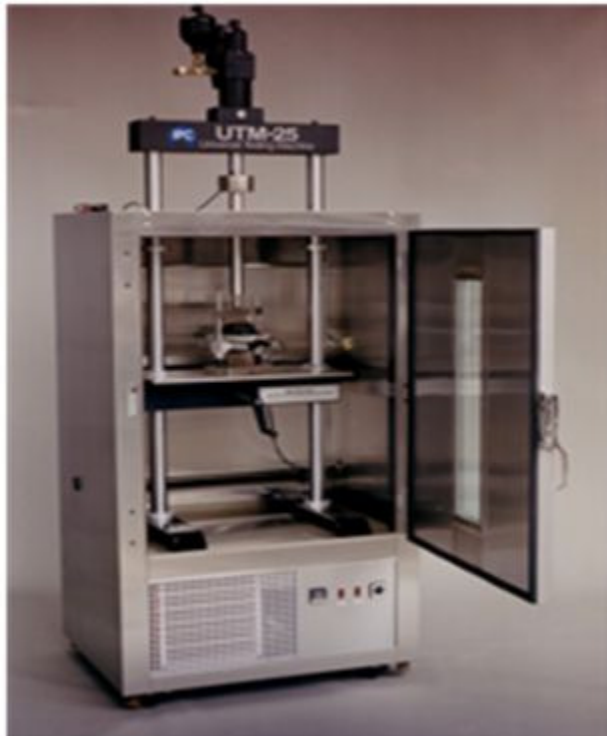
Figure 3. Indirect tensile fatigue test (ITFT) apparatus.
