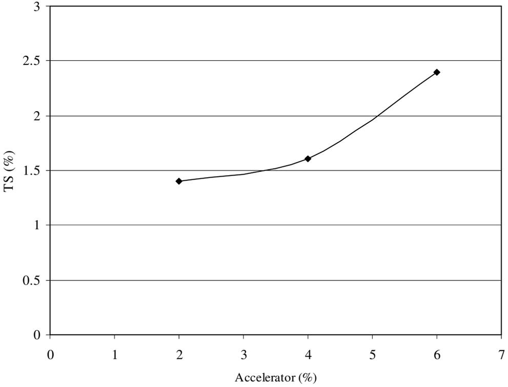
Figure 7. Effects of accelerator used on thickness swelling (TS) of the boards.
