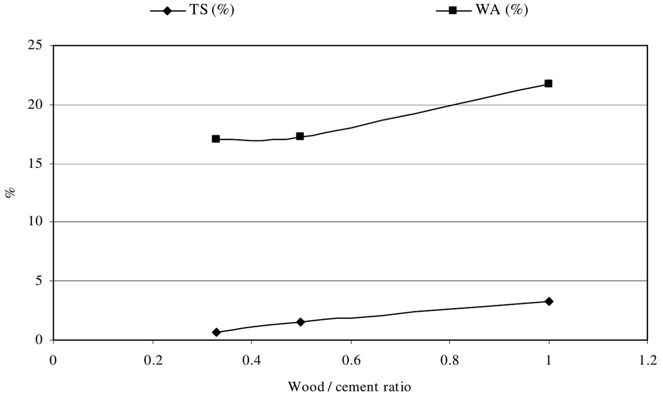
**Figure 5.** Effects of wood / cement ratio on thickness swelling (TS) and water absorption (WA) of the boards.
