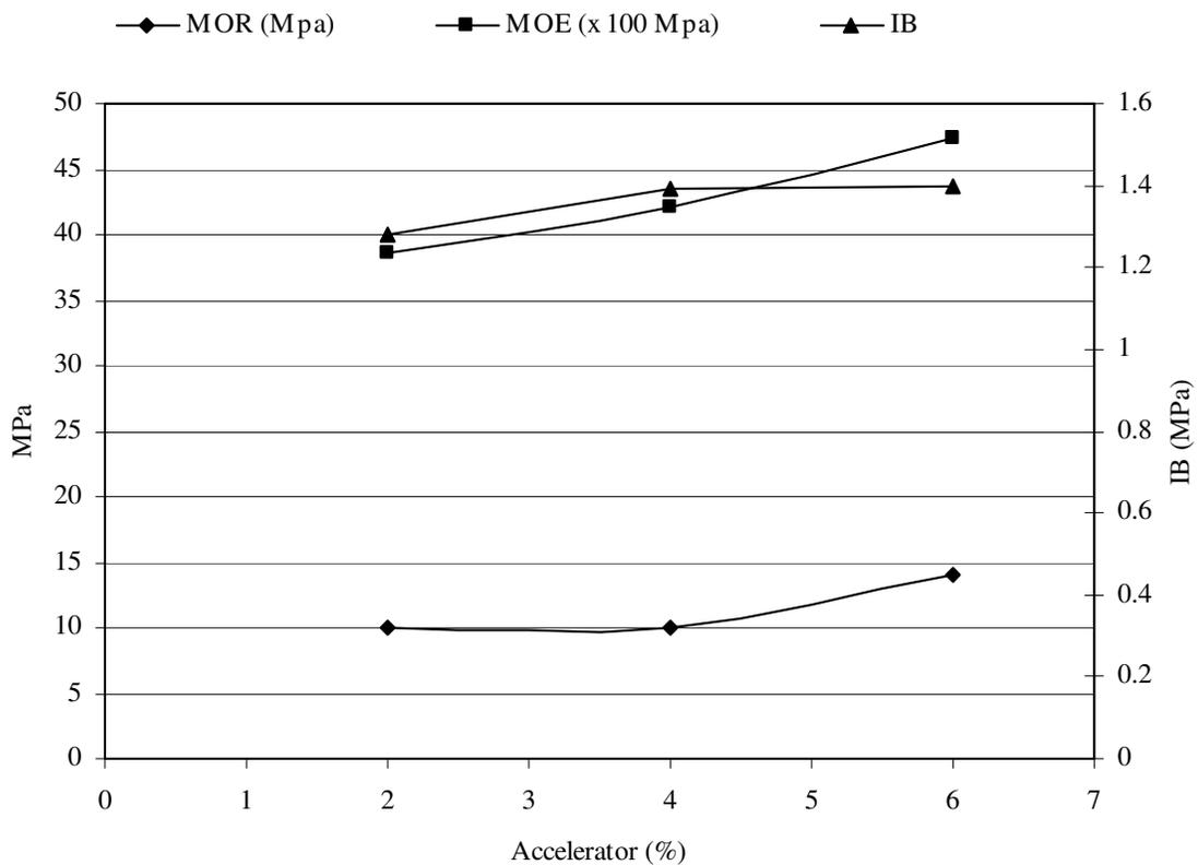
**Figure 4.** Effects of accelerator (%) on mechanical properties of the boards.
