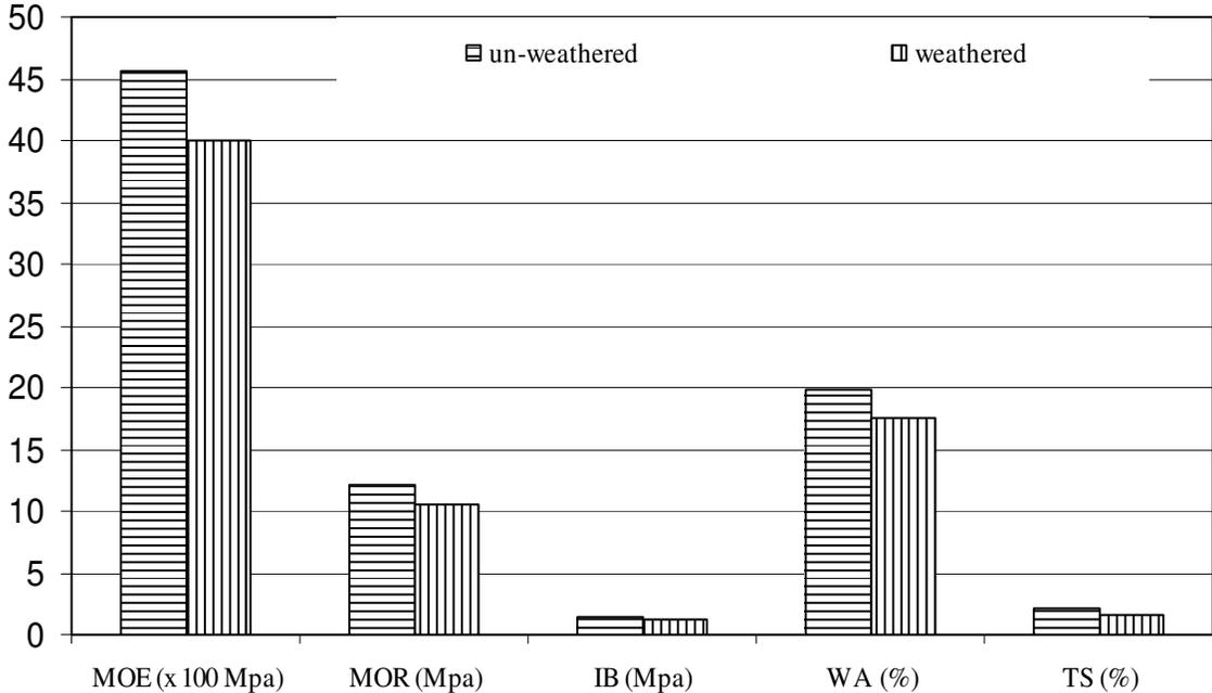
Figure 1. Effects of accelerated weathering on some physical and mechanical properties of boards.
