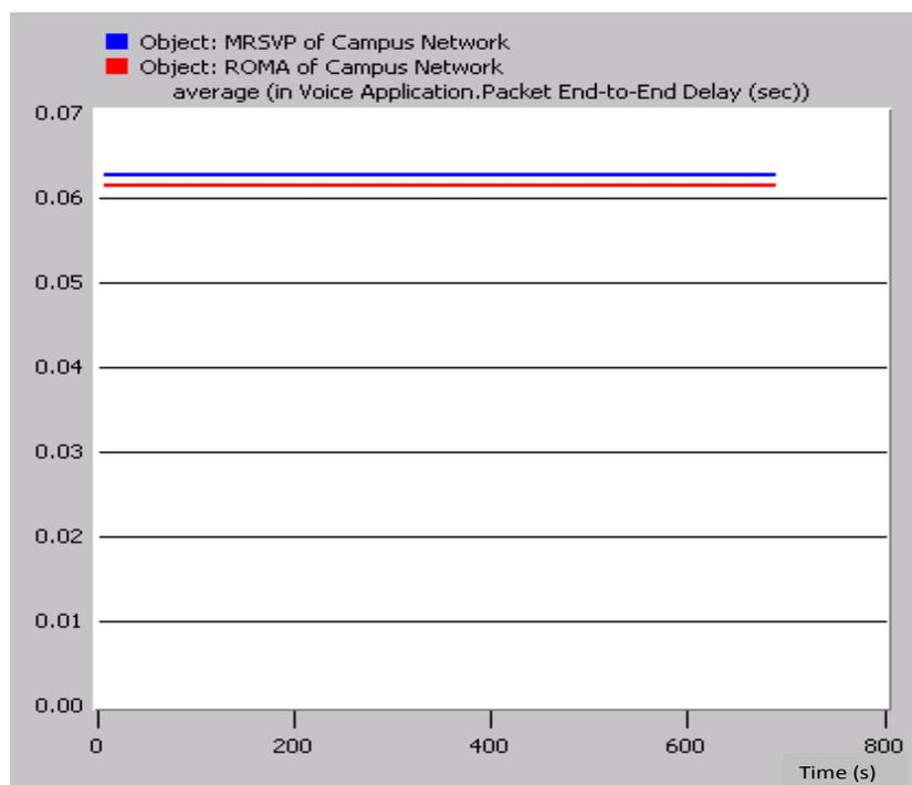
Figure 7. End to end delay for voice application.
