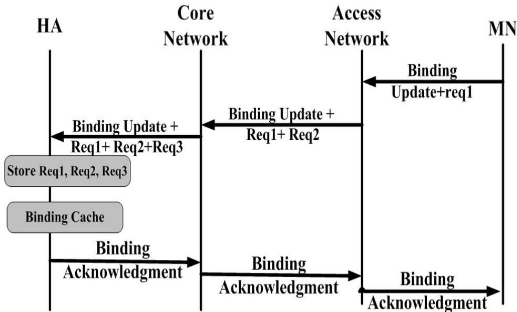
Figure 2. Modified mobility signaling for mobile IPv6.
