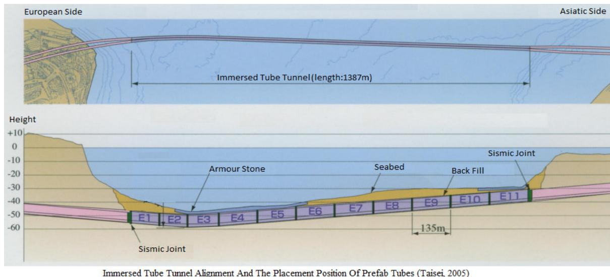
Figure 2. Immersed tube tunnel alignment and the placement of prefab tubes (Ünlütepe, 2005).
