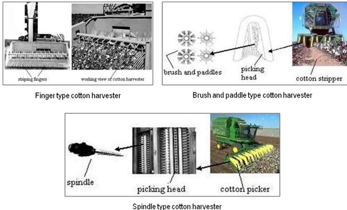
**Figure 2.** Types of cotton harvesters with different mechanisms. Source: <http://www.cottoninc.com/fiber/AgriculturalDisciplines/Engineering/Cotton-Harvest-Systems/Cotton-Strippers/Introduction/>.
