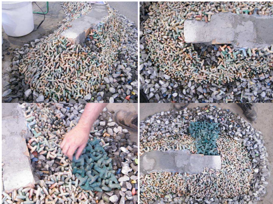
Figure 8. Breakwater Construction Images for Test 004.
