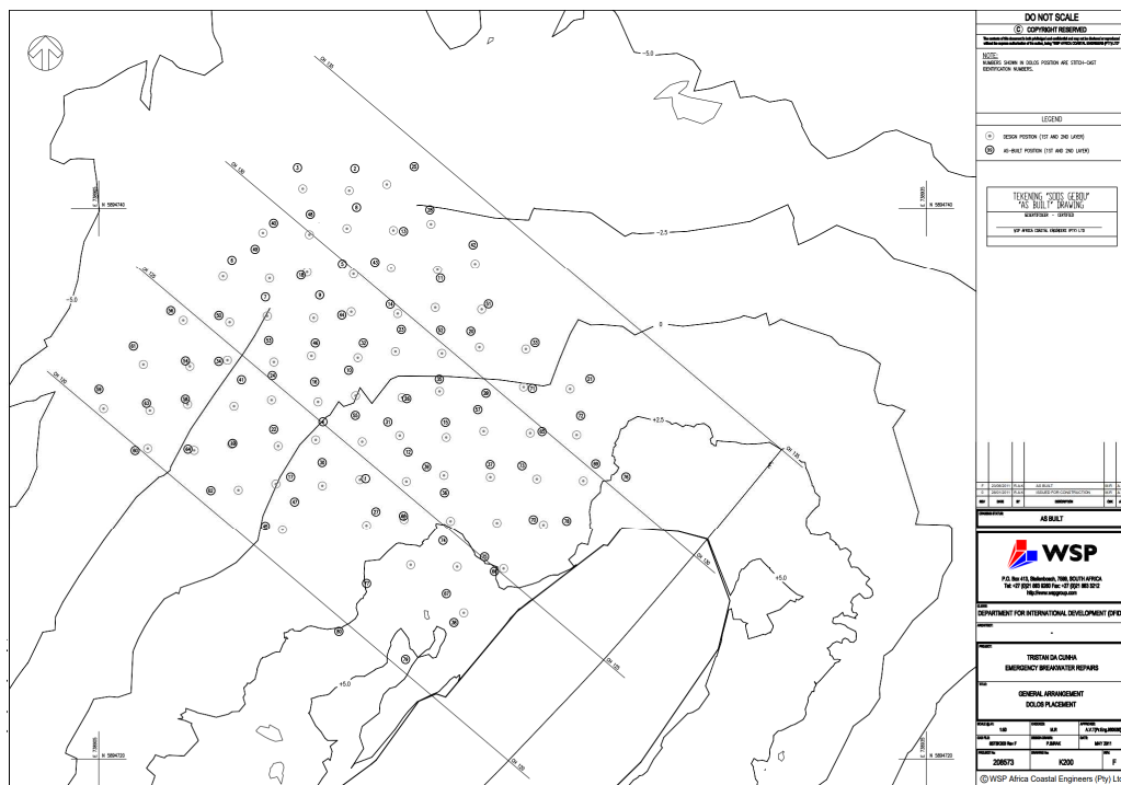
Figure 12. As-built positions of emergency repair dolosse.
