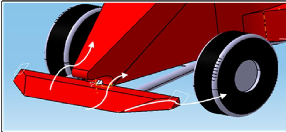
Figure 10. Air flow on front wing.
