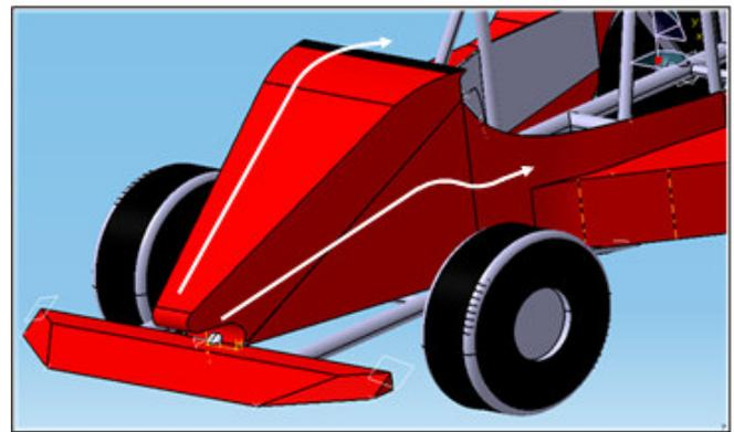
Figure 12. Air flow on nose.
