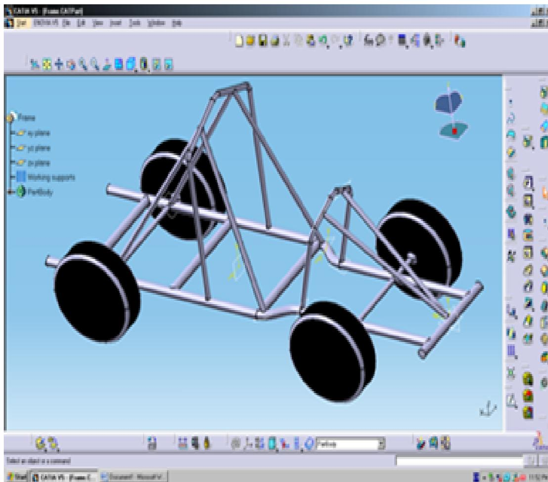
**Figure 3.** 3D solid model of the chassis.
