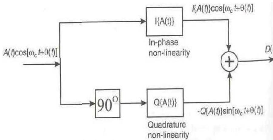
Figure 2. Cartesian form of envelope nonlinearity for AM/AM and AM/PM.
