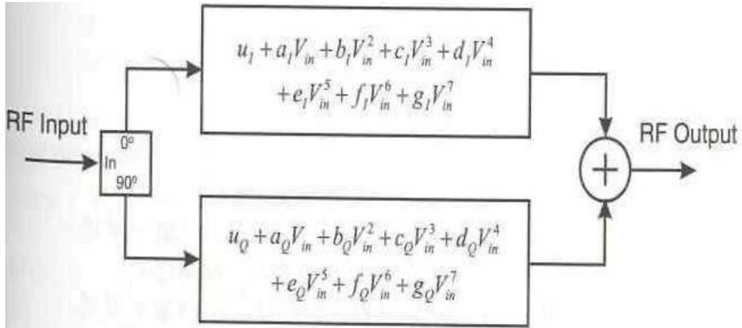
Figure 4. Diagrammatic representation of power series
