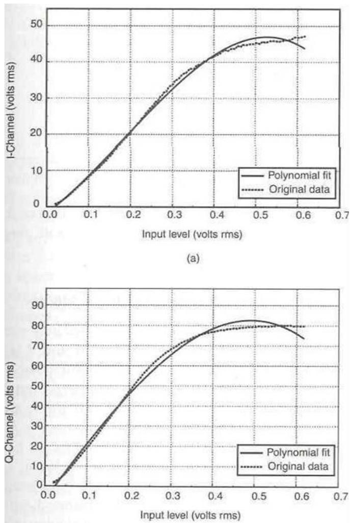
**Figure 3.** Cartesian form of envelope characteristics for a Class C amplifier.
