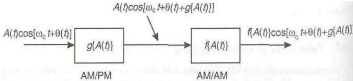
Figure 1. Polar form of envelope nonlinearity for AM/AM and AM/PM distortion.
