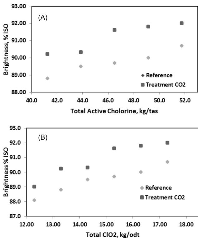
**Figure 2.** (A) Amount of total active chlorine, kg/odt necessary to achieve a given brightness, the  $D_1$  stage being conducted at pH 4.0 (reference), and 5.5 (buffered with  $\text{CO}_2$ ); (B) Amount of chlorine dioxide required to reach a brightness of 90% ISO kg/odt;  $D_1$  stage being conducted at pH 4.0 (reference), and 5.5 (buffered with  $\text{CO}_2$ )
