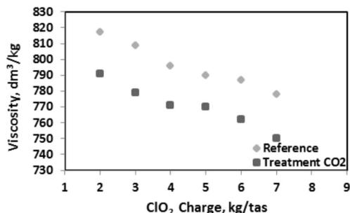
**Figure 5.** Final viscosity of the pulps bleached by conventional procedures (reference), and buffered with chlorine dioxide at a pH near neutral (the chlorine dioxide neutralized)
