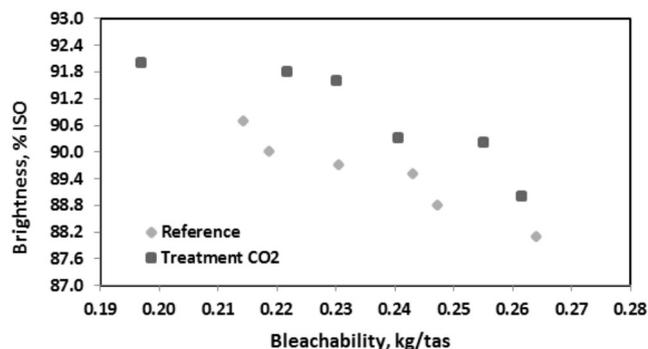
**Figure 3.** Bleachability kg/odt a bleached eucalyptus kraft pulp with a sequence  $D_0(\text{EP})D_1$ , obtained in different brightness bands, the  $D_1$  stage being conducted at pH 4.0 (reference), and 5.5 (buffered with  $\text{CO}_2$ )
