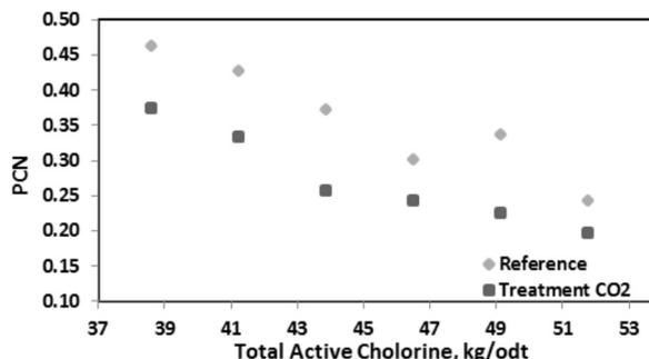
**Figure 4.** Brightness stability as measured by post color number (PCN), the pulps bleached by the conventional method (reference), and chlorine dioxide at near neutral pH (buffered with  $\text{CO}_2$ )
