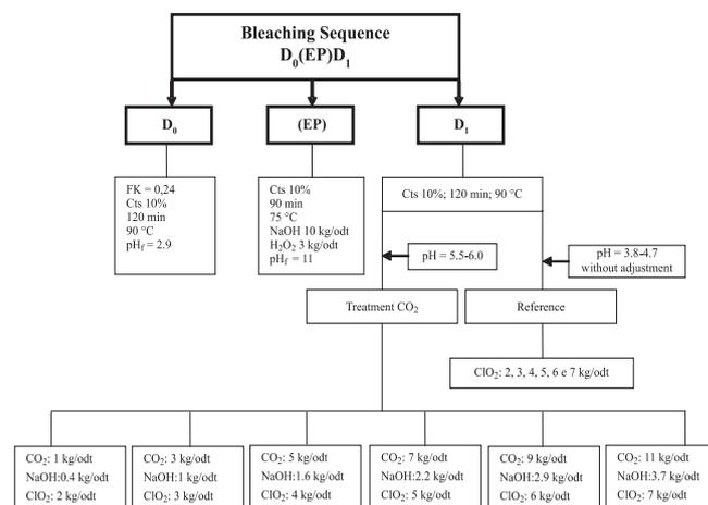
Figure 1. Experimental design of the investigation of using ClO<sub>2</sub> near neutral
