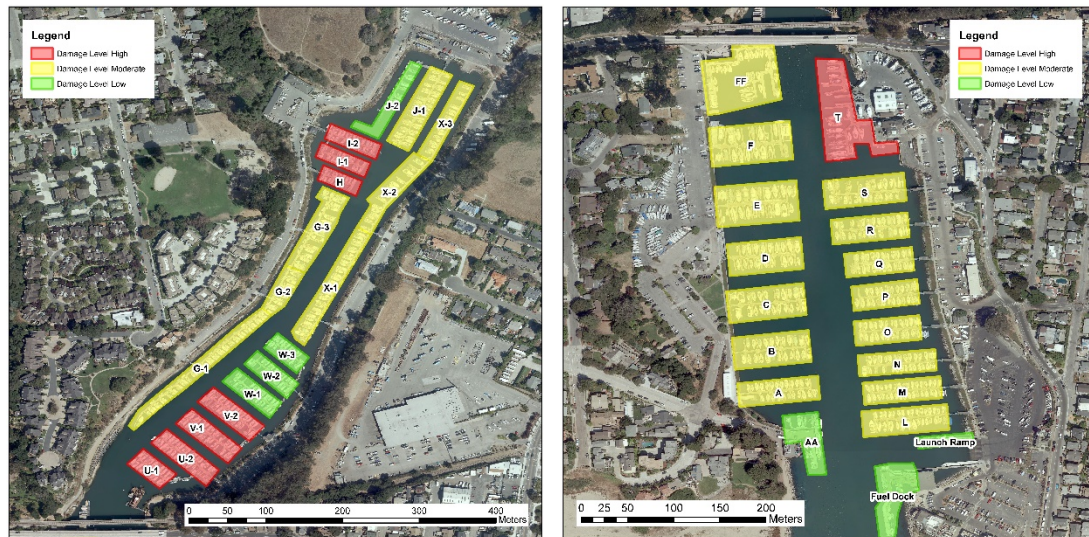
Figure 2. Damage survey of the Santa Cruz Harbor north (left) and south (right) basins showing areas of high (red), medium (yellow) and low (green) slip damage.
