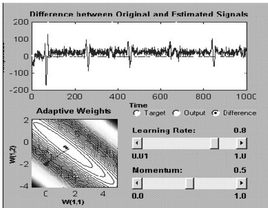
Figure 8. Difference signal (fetal ECG) of network in noisy environment.
