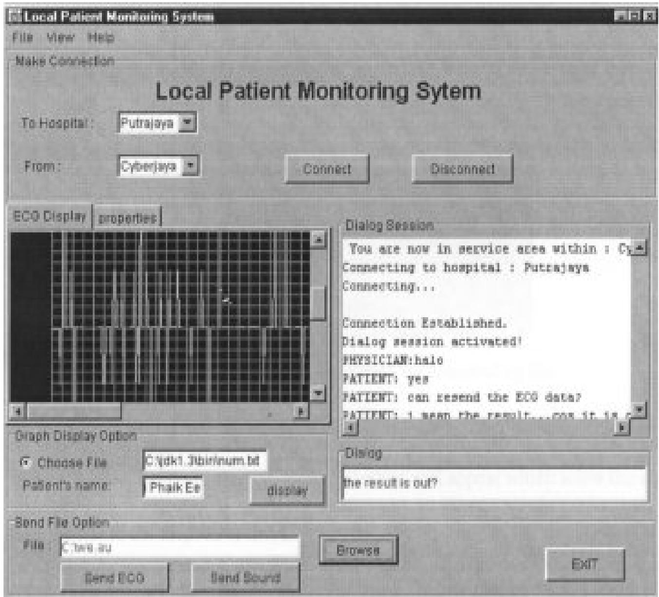
Figure 6. Graphical user interface for using features at LPMS.
