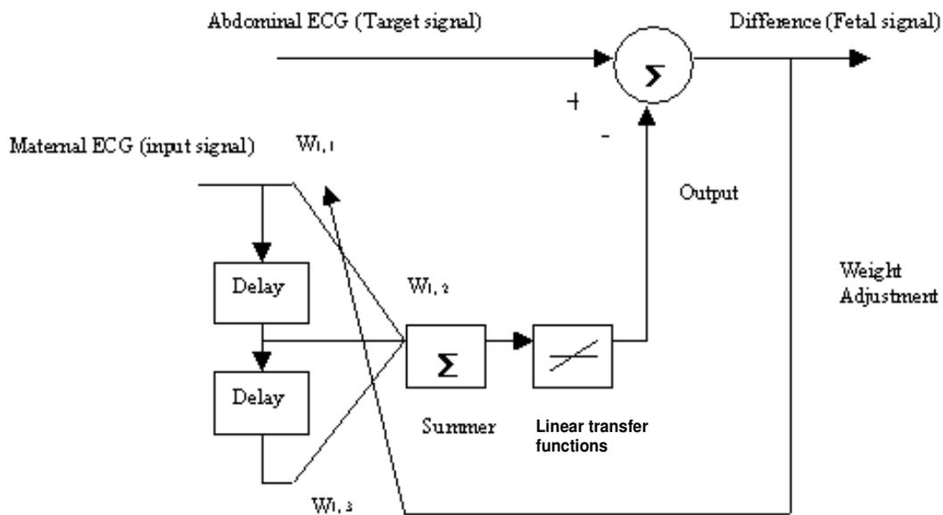
**Figure 1.** Adaptive linear neural network filter architecture.
