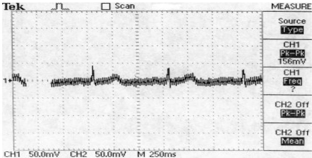
Figure 4. The amplified ECG signal from the instrumentation amplifier after feeding it into a high pass filter.
