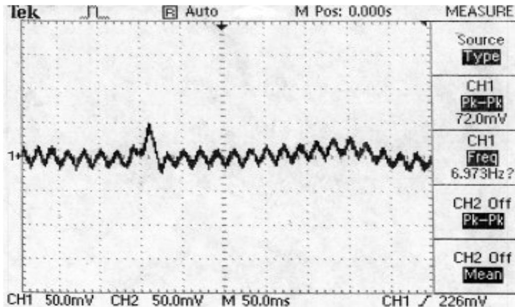
**Figure 3.** The amplified ECG signal from the instrumentation amplifier (AD620) without filtering.
