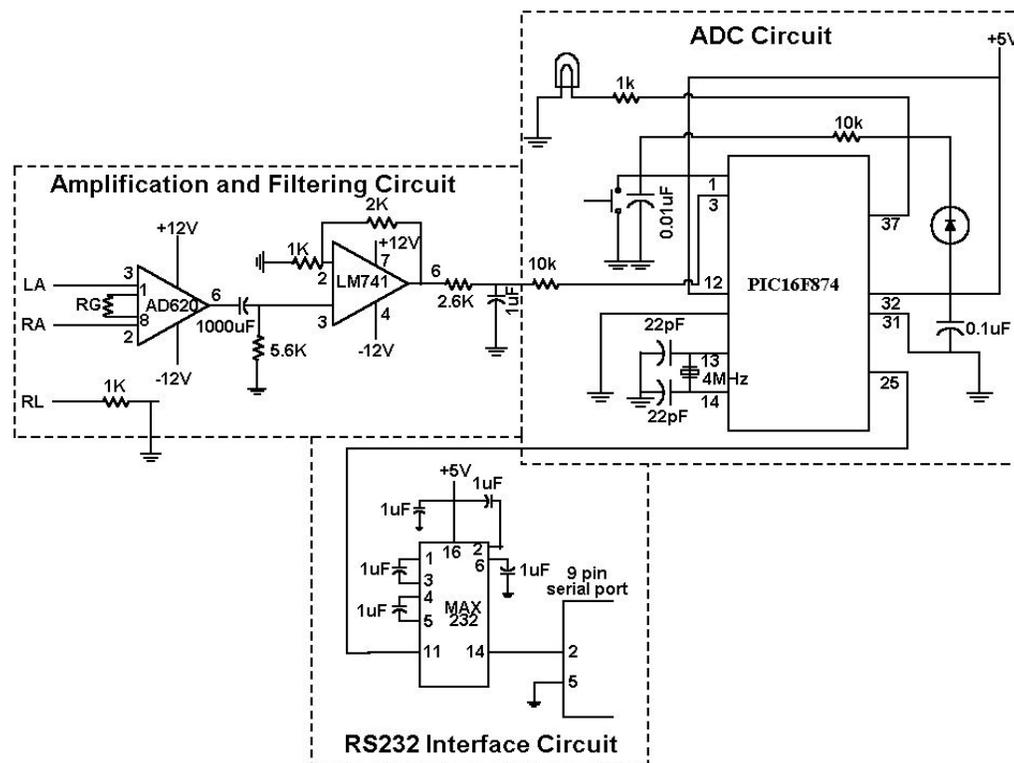
Figure 2. Schematic diagram of amplification and filtering stage.
