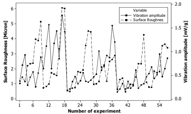
Figure 7. Time series plots of surface roughness and vibration.
