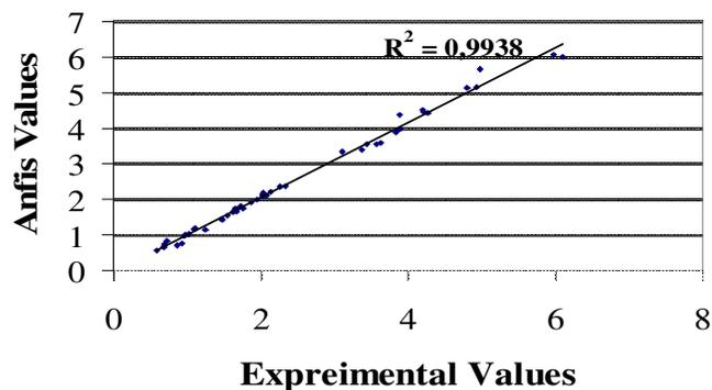
**Figure 9.** Scatter plot of the measured Ra and the predicted Ra of the ANFIS model for testing.
