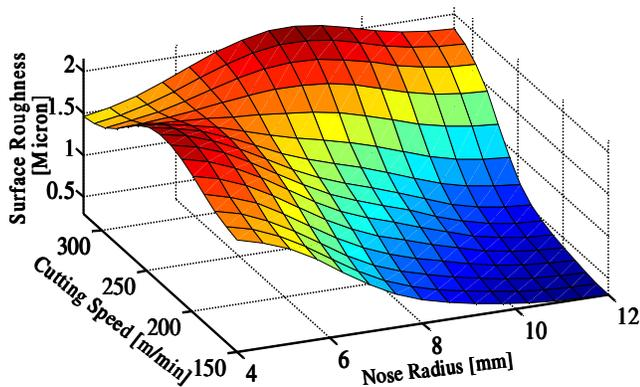
Figure 6. Effects of cutting speed and nose radius on surface roughness.
