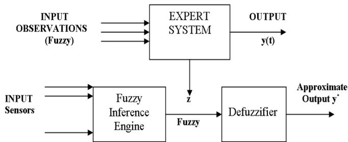
Figure 2. The basic configuration of the fuzzy system.
