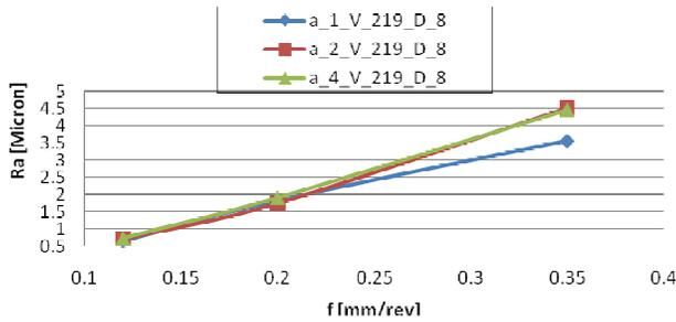
Figure 4. Effects of feed rate and depth of cut on surface roughness.
