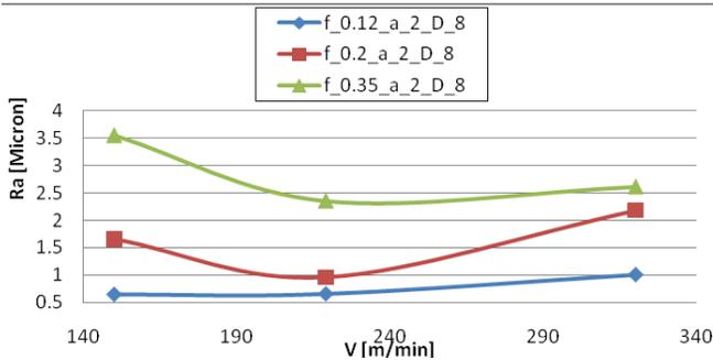
Figure 5. Effects of cutting speed and feed rate on surface roughness.
